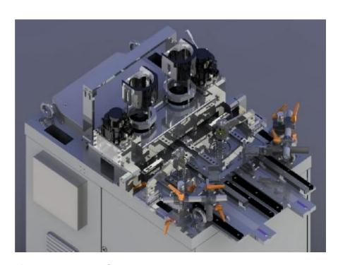
Ends are fed through an infeed hopper to 3 Cam Rollers separators, driven by with min/max height sensors.
